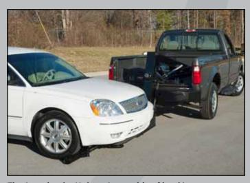
The Snatcher by Holmes is capable of hooking up to a vehicle at a 90° angle, such as parallel parked vehicles.
