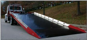
The innovative SST<sup>TM</sup> option provides a Solid Sloped Tail section that improves the load angle by 3 1/2 degrees.
