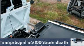
The unique design of the SP 8000 Sidepuller allows the operator to use the removable sheave head on either side or winch directly from the center pivoting sheave. The center sheave is able to pivot 180 degrees, allowing you to winch in any direction behind the cab, even straight onto the carrier deck.
