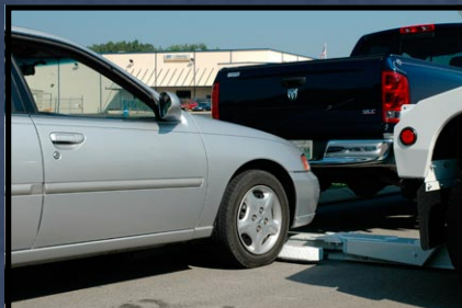
As the low profile crossbar contacts the side of the tire it pivots around into position in front of the tires.
