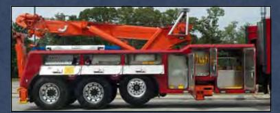
Century's aluminum body is designed to optimize space for your lift forks and popular towing and recovery equipment. Optional front tunnel saddle boxes are available in a variety of sizes to meet your specific equipment needs. All Century bodies come with an aluminum tread-plate walkway for easy access to the center section of the recovery unit.
