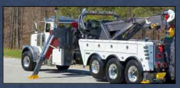
The new Century RXP option for the 1130 and 1140 tri-axle rotators incorporates dual 35,000-lb., two-speed planetary winches, as well as 212" of spread for more stability when lifting. The RXP also provides additional front-axle weight for towing heavier loads and gives operators countless rigging possibilities for those difficult recoveries, thanks to the two additional winches.
