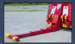
The LDU is standard on both the 1130 and 1140, and provides 136" of reach with a lift capacity of 15,000 lbs. when fully extended. Fully retracted, the LDU has a reach of 51" and a lift capacity of 35,000 lbs.
