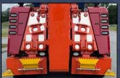
The rear outriggers on the Century Rotators were redesigned with a 2½° angle and are now fitted with new lighter-weight spade attachments that are easily stored on the rear legs. The user-
