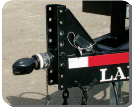
The hitch adjusts from 12" to 24" vertically.
