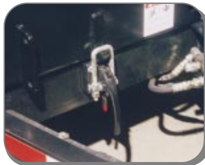
A heavy duty bed lockdown with safety latch firmly secures the bed in transport position.
