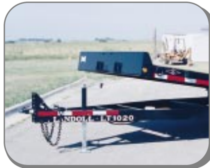
Adjustable hitch 12" to 24" vertically, plus 7,000 lb. drop leg jack are standard equipment.
