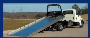
The Vulcan 10 & 15 Series Carriers are available with aluminum decks constructed of interlocking extrusions that provide durability, additional corrosion prevention, and lighter weight for increased payload capacity.
