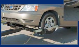
Vulcan's Strapless Wheel Retainer System is one of the easiest and safest systems on the market today. The retainers pivot both vertically and horizontally for easy hook ups in a variety of situations and best of all, no tie-down straps.
