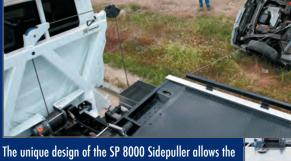
operator to use the removable sheave head on either side or winch directly from the center pivoting sheave. The center sheave is able to pivot 180 degrees, allowing you to winch in any direction behind the cab, even straight onto the carrier deck.
