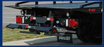
The low profile fabricated wheel-lift stinger provides 68" of reach. When retracted the crossbar is tucked in close to tailboard with minimal overhang. Vulcan's Strapless Wheel Retainer System or the popular AutoGrip II crossbar is also available.
