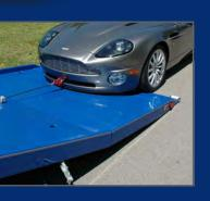
After the vehicle's front wheels are on the carrier, the deck can be leveled out and the cable guide removed allowing the vehicle to overcome the second clearance problem with the forward section of the deck. With the front wheels on the front section of the deck the process can be repeated again to eliminate clearance problems such as low exhaust or extended rear overhang.
