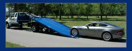
The Extreme Angle option available on Vulcan 10 series steel carriers eliminates the need for wood planks or ramps when loading and unloading low clearance vehicles. The release handle allows the rear hinged deck section to be lowered to a 6° load angle. A removable cable guide is inserted in the deck to keep the cable low while winching the vehicle onto the rear deck.
