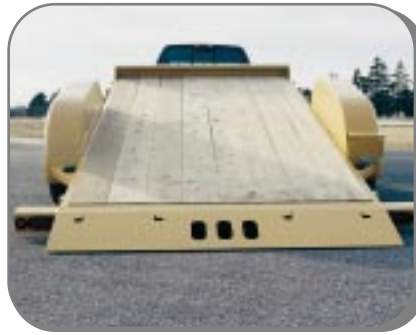
A full width rear light bar for added safety protection with machined safety approach plate.
