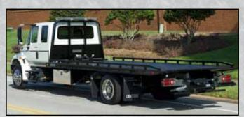
When mounted on most air ride chassis, with the air dumped, the 16 series L.C.G. has lower then an 11° load angle, making it ideal for loading low clearance vehicles or equipment without using ramps or wood.
