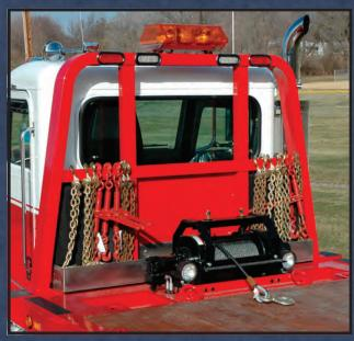
The optional steel tube cab protector includes a rack for your chains and binders. Steel wire mesh can be added for additional protection of the rear window. A stainless steel chain tray is available for the stationary cab protector.
