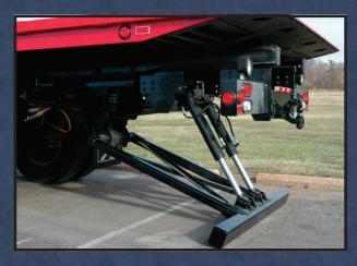
A hydraulic dock stabilizer is standard on all 30 Series carriers, and is available in lieu of the wheel lift on the 20 Series carrier. Century's mounting plate above the stabilizer accommodates the optional pintle hook.
