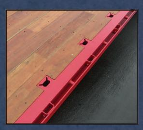
The optional outside stake pockets with rub rails and pipe spools can be combined with additional key slots to provide more versatile tie-down options.
