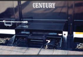
The 20 Series carrier comes standard with an 8,000-lb. worm gear winch. The optional 12,000-lb. planetary winch is shown here with the optional winch cover and 4-way roller guide.
