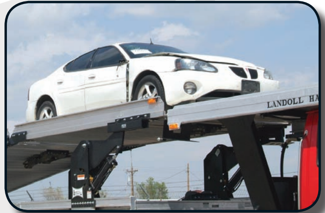
❖ The Adjustable Upper Deck Allows for Easy Transition from Trailer to Overcab
