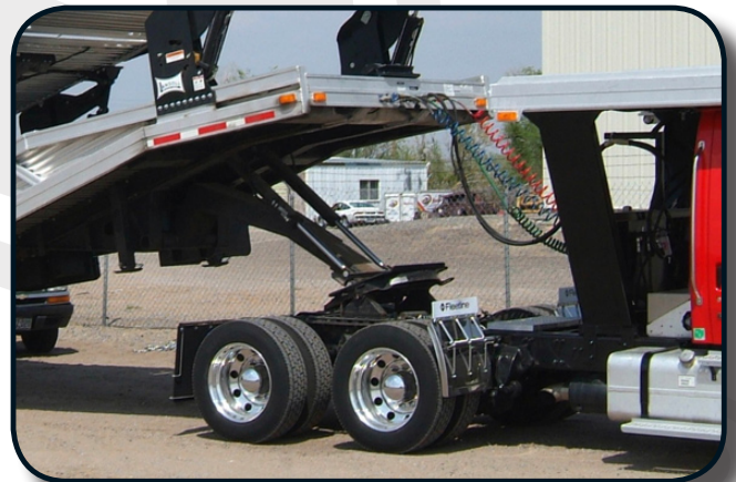
❖ Tilt Cylinder - Major Steel Components Powder Coated
