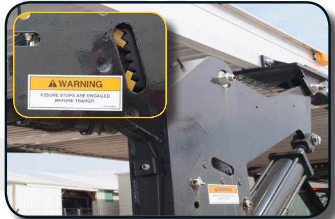
❖ Hydraulic Adjustable 24" Vertical Travel
