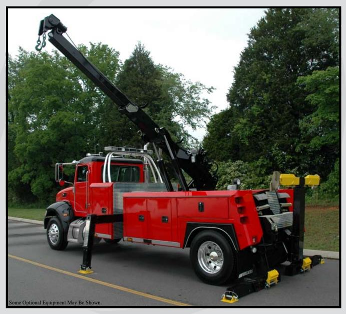
Holmes opens up a whole new dimension in medium duty towing and recovery with the Holmes 600R. A recovery boom with 16 tons of retracted capacity and 6 tons of extended capacity that rotates 220° makes this the most versatile unit yet from the oldest and most trusted name in the industry. The underlift with 89" of reach easily handles a wide range of vehicles from autos through trucks. Visit your local Holmes distributor to learn how the Holmes 600R can increase your bottom line.
