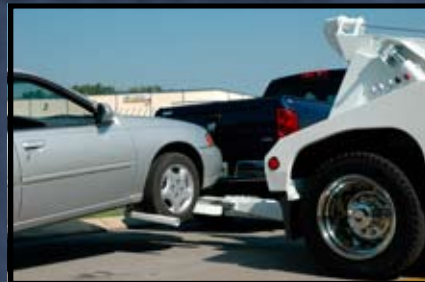
The operator now closes the arms around the tires and raises the vehicle without ever getting out of his truck. The operator is now ready to exit his truck and install the proper safety equipment.
