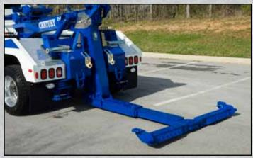
The fabricated underlift is rated at 7,000 lbs. lift capacity at its fully extended reach using lifting forks and has a tow capacity of 20,000 lbs. This makes the Century 2465 ideal for towing a wide variety of light- and medium-duty trucks, as well as automobiles.
