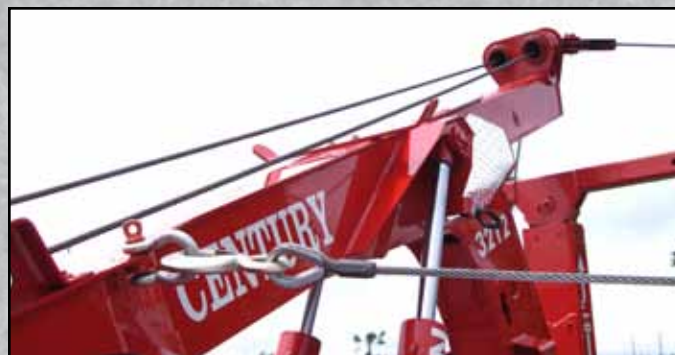
The 3212 allows the cable to be run through a snatch block and hooked to a clevis at the base end of the boom for side pull applications.
