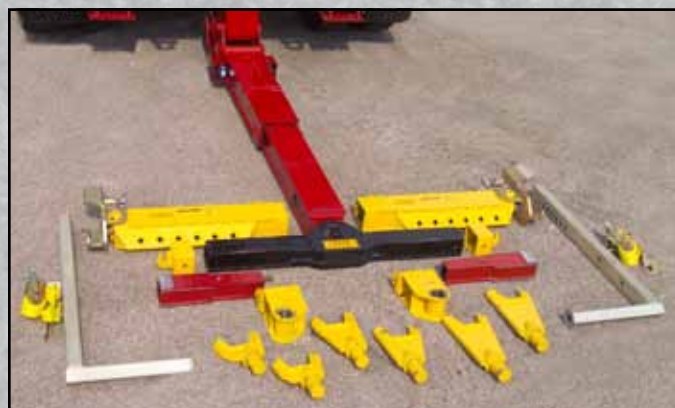
The 3212 comes standard with a low-profile crossbar with removable ends, 3 sets of lift forks, fork holders and a 6,000-lb. pivoting L-Arm System
