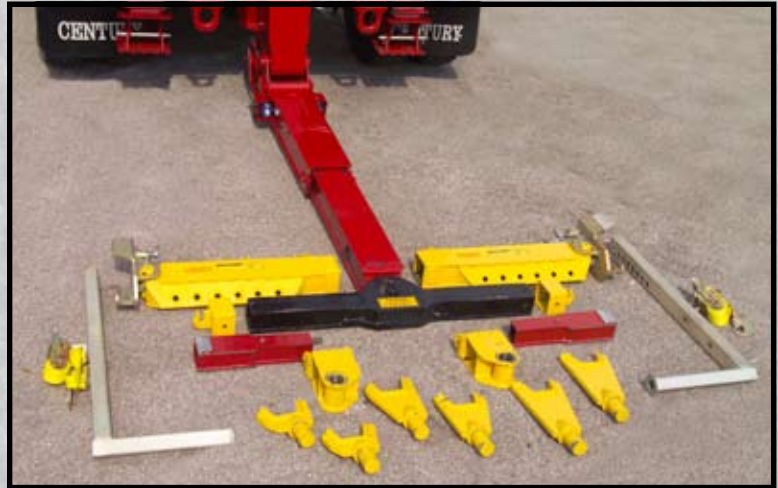
The 3212-CX2 comes standard with a low profile crossbar with removable ends, 3 sets of lift forks, fork holders, and 6,000 lbs. pivoting L-Arm System.
