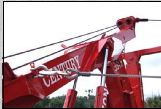
The 3212-CX2 allows the cable to be run through a snatch block and hooked to a clevis at the base end of the boom for side pull applications.
