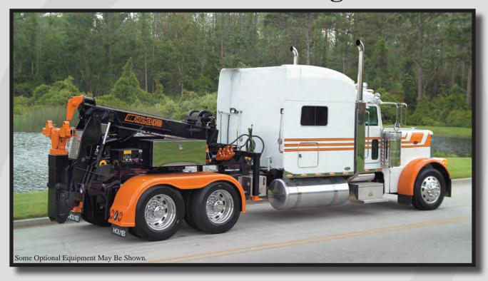
The new Holmes D.T.U. (Detachable Towing Unit) offers proven design and technology from the oldest and most trusted name in the towing industry. The front legs allow the unit to be easily removed in a matter of minutes so your truck can be multifunctional for both towing or pulling trailers.
