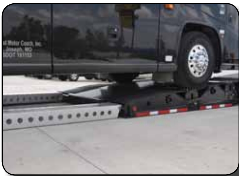
The Mechanical Wheel Well Lifter Allows the Bus to Smoothly Transition Over the Rear Wheel Wells.
