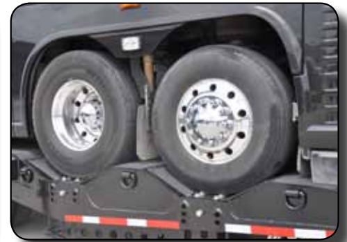
Adjustable Wheel Well Pockets with Five Different Positions Minimizes the Clearance Under the Bus as well as Lowers the Overall Height.
