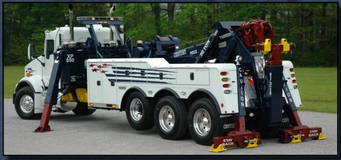
All recovery operators have experienced the problems of having traffic backed up with a casualty down in a ravine and the law enforcement not wanting to block lanes of traffic. The SP 850-XP option can solve these types of situations with a pivoting hydraulic stiff-leg to handle tough side pull recoveries and eliminate the need to block more lanes of traffic than necessary.
