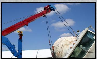
The SP 850-XP allows the operator to run the two winch cables from the XP unit to snatch blocks on the boom, allowing a total of four winch lines to be utilized for recoveries off the tailboard. In this scenario doing a reverse roll, two winches are used for the lift while the other winches are utilized as the catch lines eliminating the need for an additional unit.
