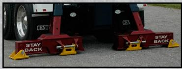
The optional rear stabilizers, similar to those used on Century Rotators, provide hydraulic horizontal extension of up to an additional 48" of stance when extended for extreme side pull recoveries.
