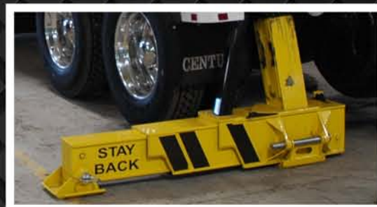
Standard three-stage rear outriggers with 174-inch stance
