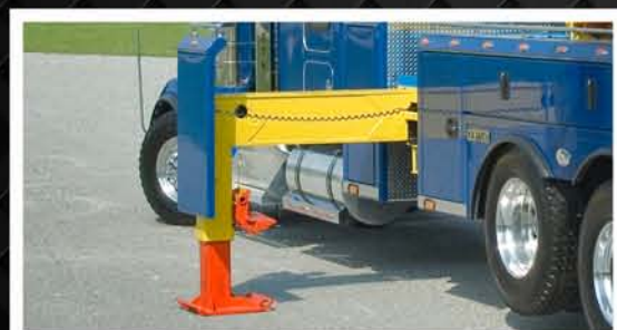
Standard top beam front outriggers with 212-inch stance
