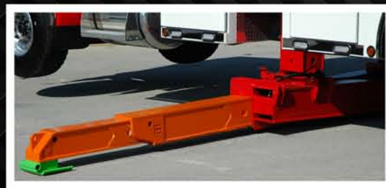
Optional three-stage front under-frame H-Beam outriggers with 262-inch stance
