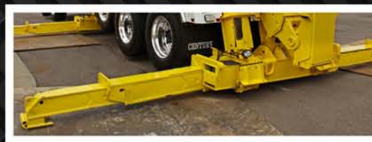
Optional rear H-Beam outrigger with 262-inch stance (requires HHU underlift in place of SDU-4)
