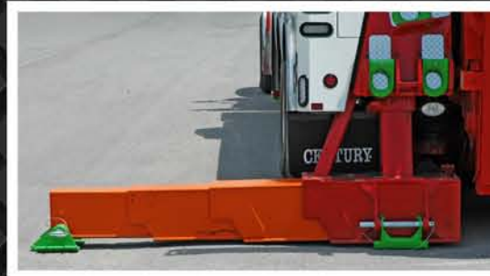
Optional four-stage rear outriggers with 220-inch stance
