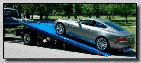
The Extreme Angle option provides you with the versatility of having a straight carrier deck with the added benefit of an angled approach plate only when you need it for exotic or low clearance vehicles.
