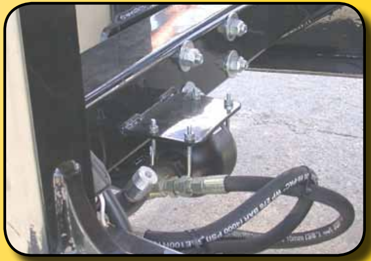
❖ Accumulator and Valve
