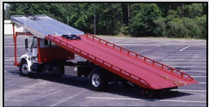
The deck over the cab tilts hydraulically for easy loading and unloading.
