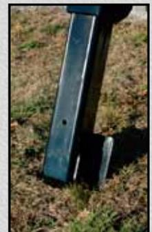
The swivel feet may be used as a flat pad for hard-packed surfaces or the operator may flip the plunger pin and lock the pad into a spade position for softer terrain applications.
