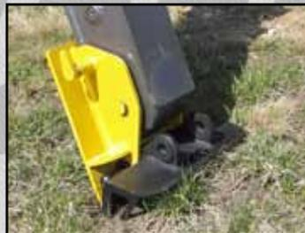
For increased holding power in the dirt or ground, the optional spade attachment provides more bite during those difficult recoveries. The D-ring can also be pinned to the spade attachment for additional rigging combinations.
