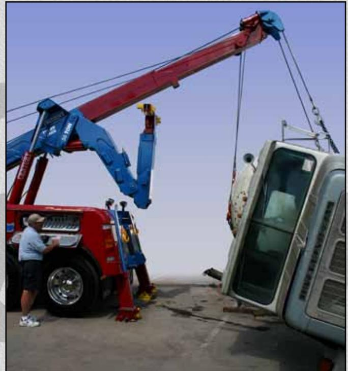
The SP 850-XP allows the operator to run the two winch cables from the XP unit to snatch blocks on the boom allowing a total of four winch lines.
