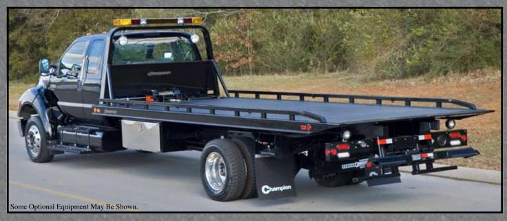
Champion car carriers are the most unique in the industry because they were designed not only for the customer but by the customer. Champion surveyed operators asking what features the ideal carrier would incorporate. The result was the Champion carrier, designed for easy maintenance and durability with features such as full length nylatron wear pads, a heavy duty subframe, full width rear pivot pin and a full height steel cab protector.
