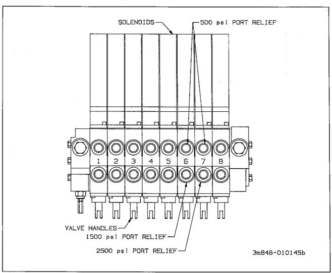
Figure 4-2 Pressure Settings for Control Valve Ports
