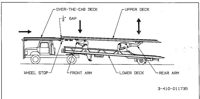
Figure 3-7 Lining Up the Over-the-Cab Deck
