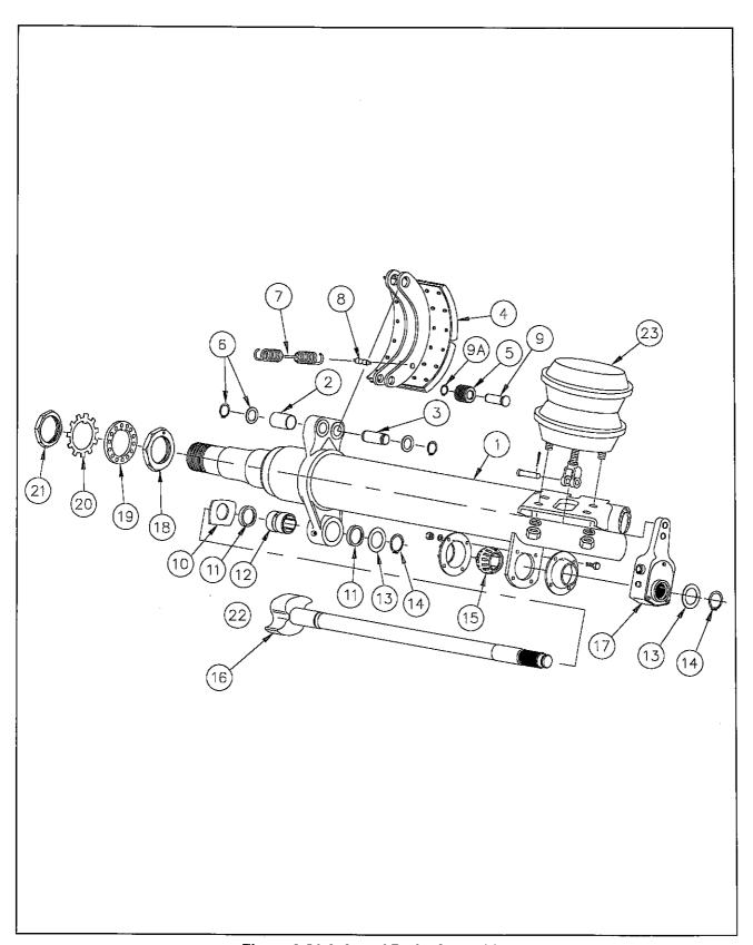
Figure 6-21 Axle and Brake Assembly
