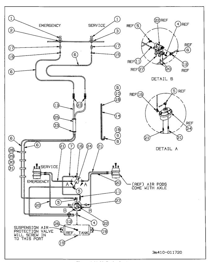
Figure 6-23 Air Brake System
