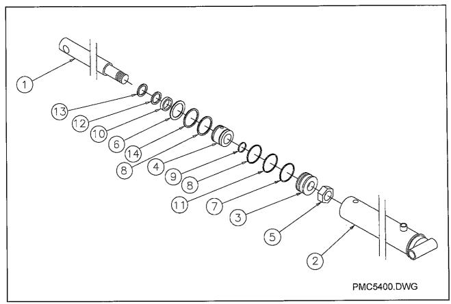
Figure 6-37 Hydraulic Cylinder 3" X 48"
