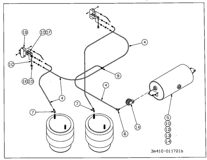
Figure 6-20 Air Ride Suspension System
