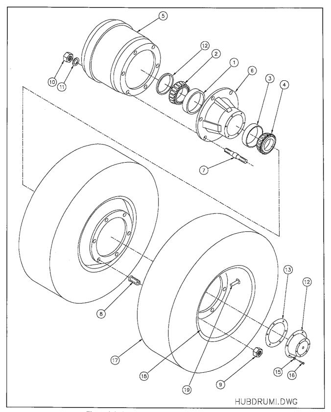
Figure 6-24 Inboard Ball Seat Mount Hub and Drum
