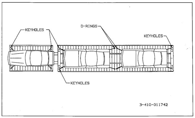
Figure 3-12 Securing the Load
