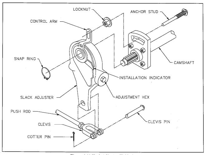
Figure 4-11 Slack Adjuster (Haldex)
