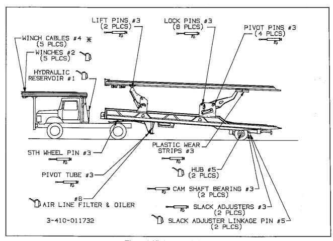
Figure 4-1 Lubrication Points
