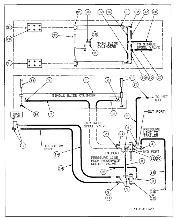
Figure 6-36 "Over-the-Cab" Hydraulic System
