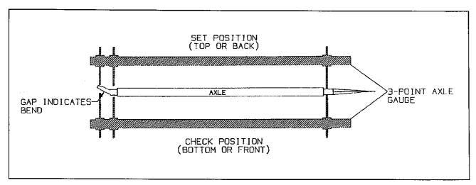
Figure 4-5 Checking Axle for Bend
