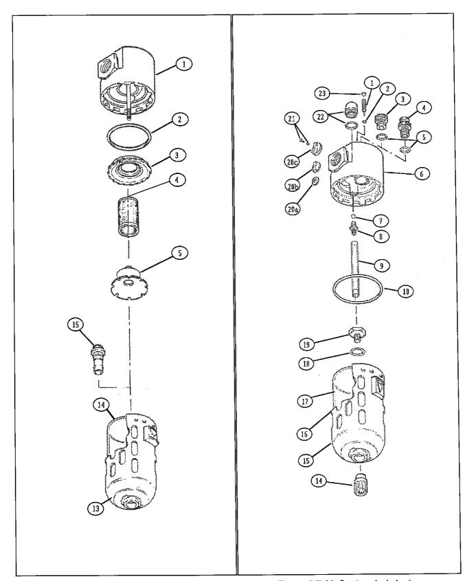
Figure 6-6 Air System Filter
