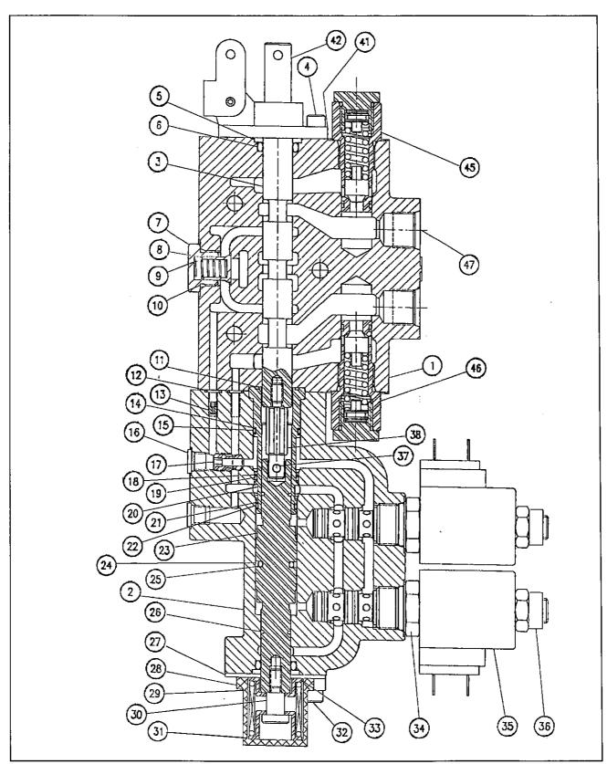
Figure 6-15 Eight Spool Valve, Work Sections (SVA-S61 shown)
