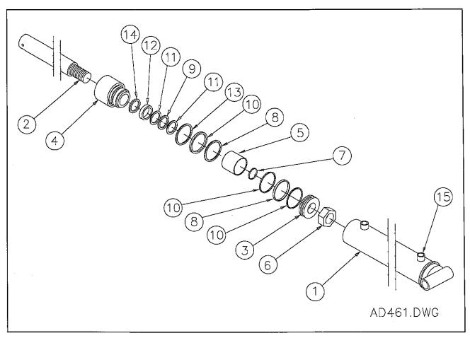
Figure 6-13 Hydraulic Cylinder Assembly
