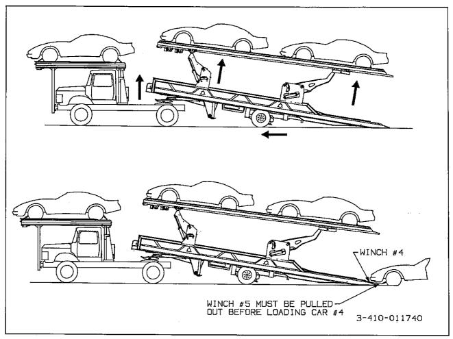
Figure 3-10 Preparing to Load the Lower Deck
