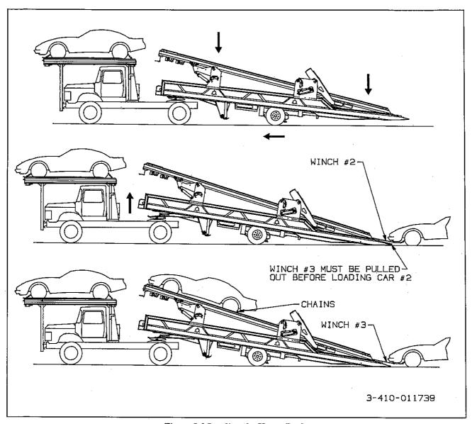
Figure 3-9 Loading the Upper Deck
