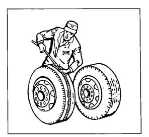
Fig. 4-17 Measuring Tape Method
